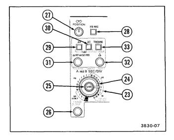
Figure 3-4. Horizontal and delta measurement controls.
