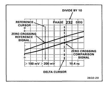
Figure 6-8. Small-angle phase difference.
