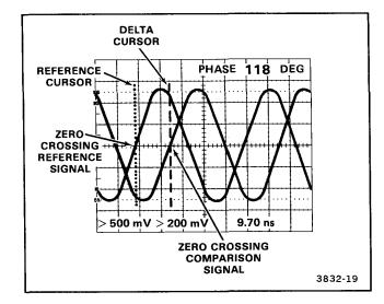
Figure 6-7. Phase difference between two time-related signals.
