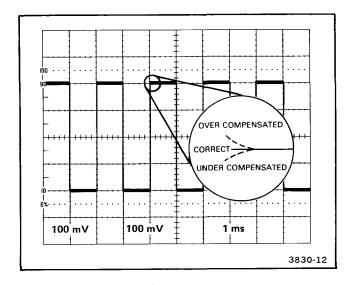
Figure 5-1. Probe low-frequency compensation.
