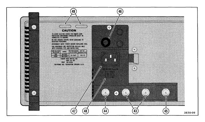
Figure 3-6. Rear-panel controls and connectors.
