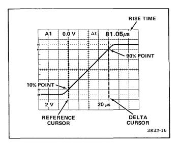
Figure 6-4. Measuring rise times.
