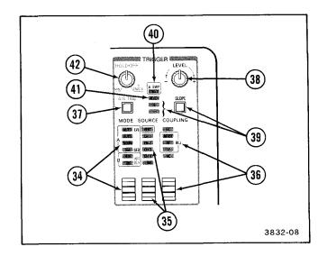
Figure 3-5. Trigger controls and indicators.
