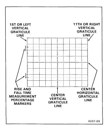
Figure 4-1. Graticule measurement markings.
