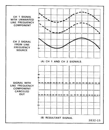
Figure 6-3. Eliminating common-mode signals.
