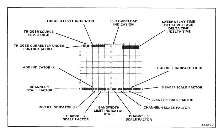
Figure 3-7. Readout display locations.
