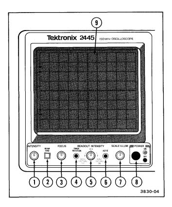
Figure 3-1. Power and display controls.
